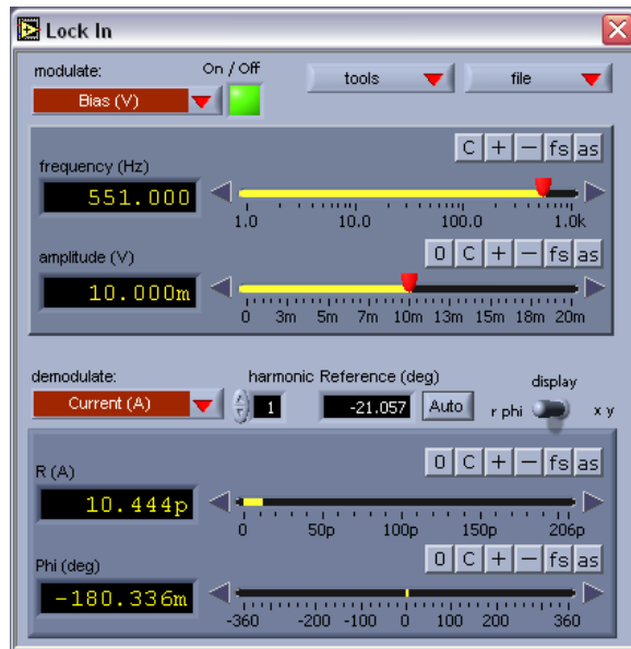
Fig.1: Screen shot of the lock-In module. The modulated and demodulated signal can be chosen from the 24 signals available in the Nanonis SPM Control System. All signals and parameters are in real world physical units.
