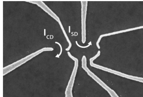
Fig. 1 Device layout with lithographically patterned gates
